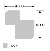
One universal profile for indoor and outdoor usage. Boards with straightcut ends can be installed without exposing the endgrain.
