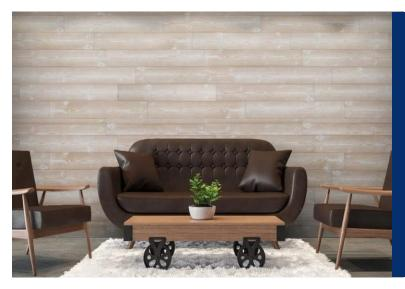
Thermory<sup>®</sup> cladding and lining in a Drift texture offers the rustic look of reclaimed timber. Thermory's spruce cladding is FSC certified and responsibly sourced from plantation timbers. Ideal for a coastal aesthetic, this blonde timber features a lime wash and delivers the performance of a thermally modified timber product, offering durability and dimensional stability.
